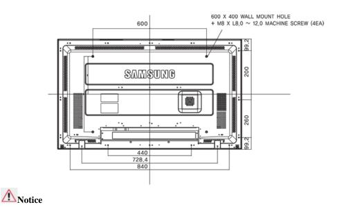
For securing the bracket on a wall, use only machine screws of 6 mm diameter and 8 to 12 mm length.
